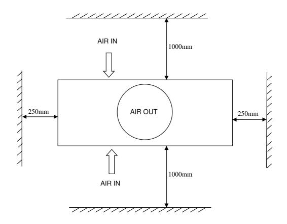
A gap of at least 1000mm is required above the dehumidifier. Appliance shall be installed, operated and stored in a room with a floor area larger than 4M<sup>2</sup>.
